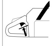
2 Press the throttle lock and make sure it returns to its original position when you release it.
